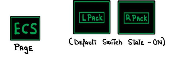
When the PIVs are commanded open the ACC ACC control their respective pack valve to modulate the ainflow based on conditions and requirements
