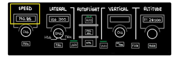
Autothrottle <u>must remain Off</u> to maintain drift down profile
