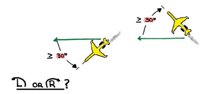
Direction of Turn is based on position of aircraft in Relation to other OTS Tracks, direction to the alternate airport, SLOP, etc.
