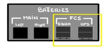
There ARE TWO (2) Flight Control System (FCS) BATTERIES:
