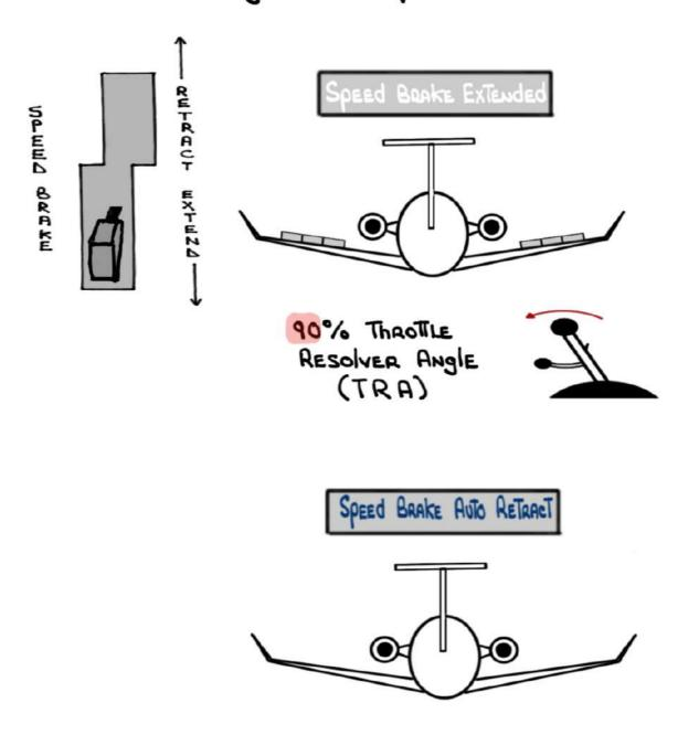
Speed brakes <u>retract</u> but speed brake handle does not
