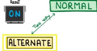
• FLT CTRL RESET Switch May allow RETURN TO NORMAL if the REASON for degrade is resolved
