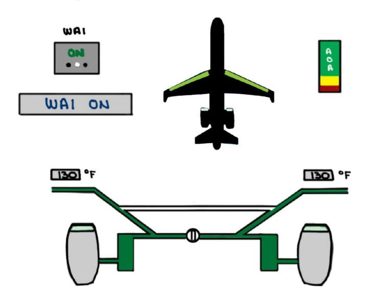
Wing TEMPERATURE MUST be > 100°F AND AIRCRAFT
