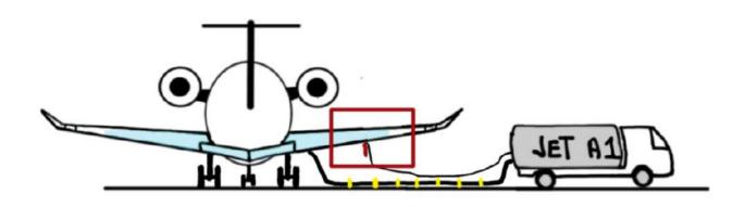
GROUNDING JACKS ARE lOCATED IN THE LOWER
