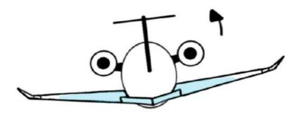
3 Open INTER TANK VALVE AND MONITOR FUEL PROGRESS
