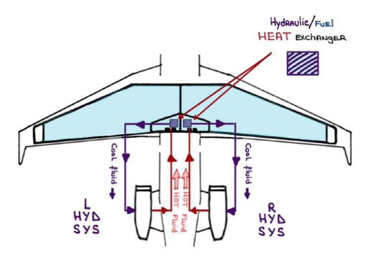
The <u>Heat Exchanger</u> unit is inside the onside fuel Hopper. HOT hydraulic fluid flows continuously Through the <u>Heat Exchanger</u> without pilot input
