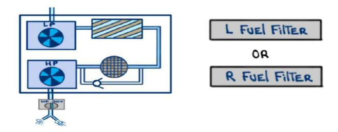
FUEL bypassing indicated filter or impending blockage bypassing of both LP filters:
