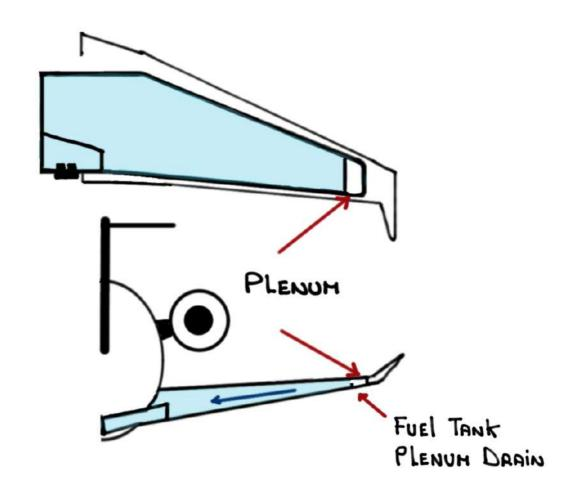
. The Plenum should be dealined of any fuel prior To Takeoff
