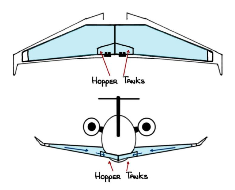
• IT is from The Hopper Tanks That fuel is drawn to feed the engines and APU
