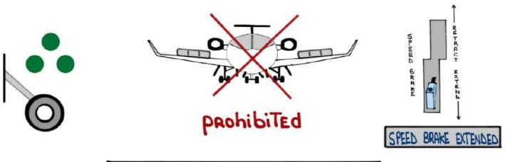
MAXIMUM TIRE SPEED: 195 KNOTS (GROUND SPEED)
