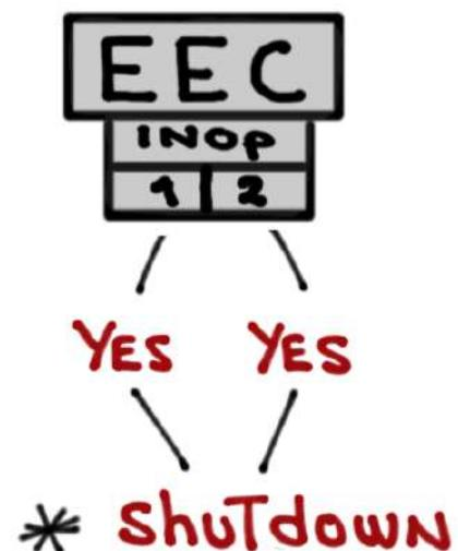
\* both CHANNELS MUST AGREE FOR TO COMMAND TO SHUT OFF FUEL TO THE ENGINE
